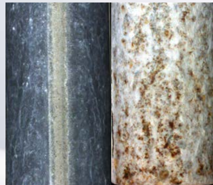
Magnelis® ZM310 welded and re-protected Post-galvanised welded
